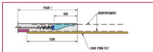
Construction Joint and Stressing Pocket
